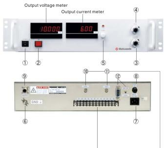
Normal Operation: Output ①→⑤, conversely to stop operation.
