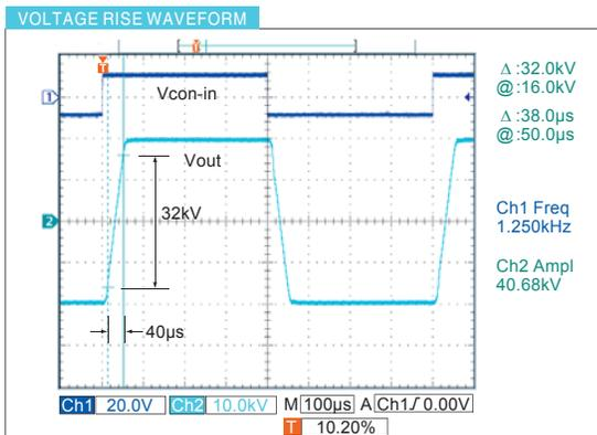
Slew rate with actual load is as high as  $700\text{V} / \mu\text{s}$ , and solve the problem of "When actual operation with load, the response become slow."
